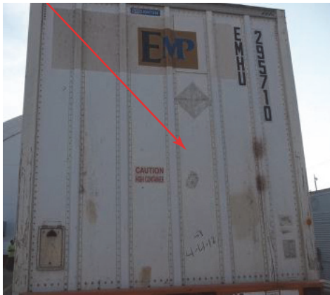
NOSE PANEL, GALVANIZED STEEL
