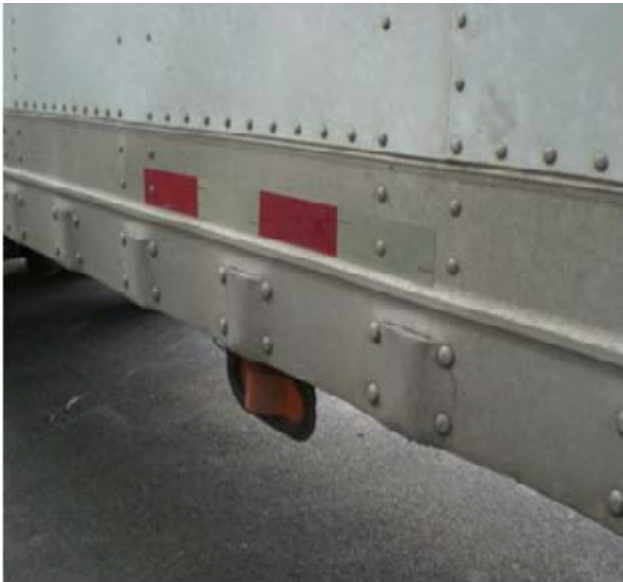
Fig. 2.6 Bottom rail deformation
