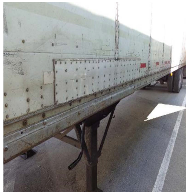
Fig. 2.34 Side panel improper repair
