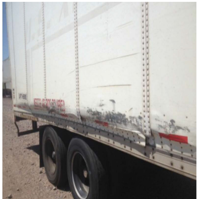
Fig. 2.30 Side panel deformation
