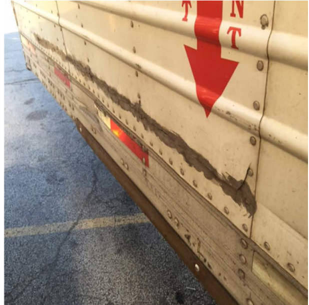
Fig. 2.28 Side panel breaks/cracks
