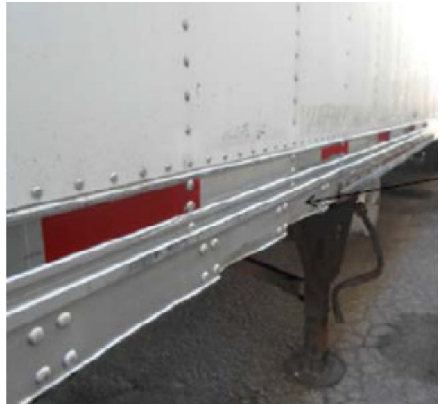
Fig. 2.7 Bottom rail deformation
