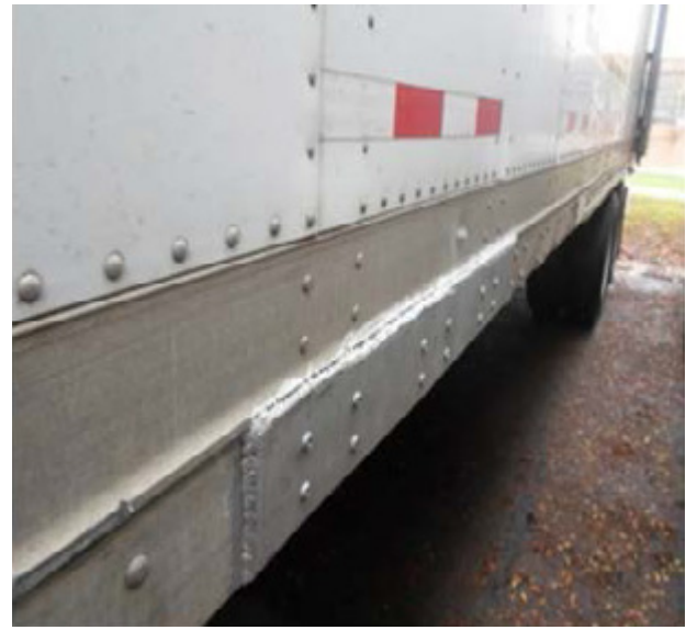
Fig. 2.15 Improper repair—welded patch
