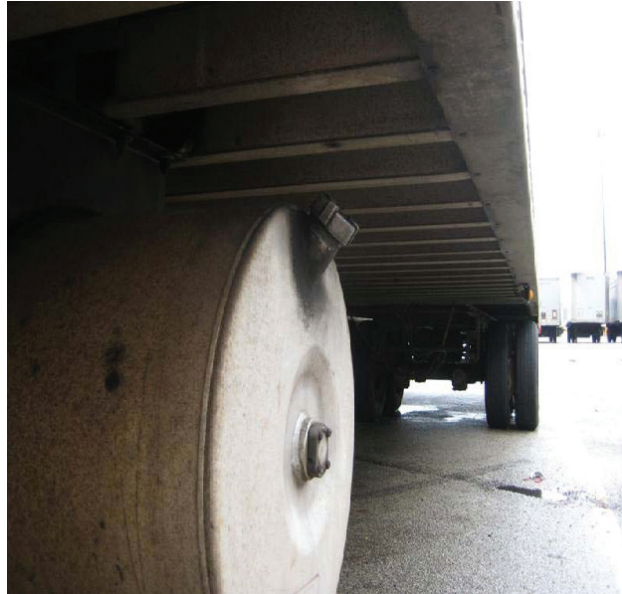
Fig. 8.1 Fuel tank properly recessed from bottom rail
