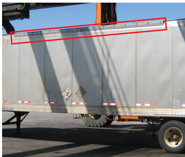
Fig. 5.1 Top rail protector—trailers longer than 40 ft
