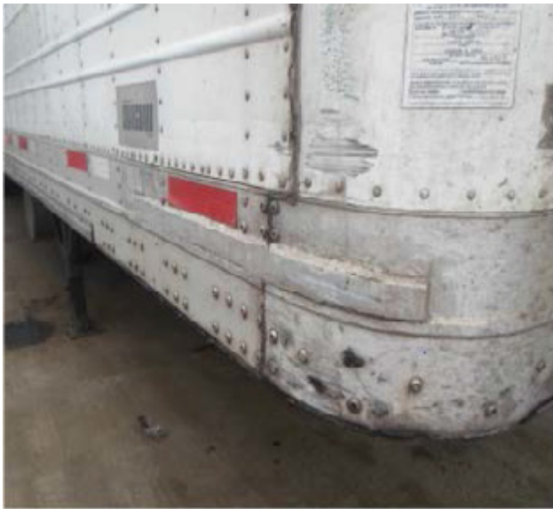
Fig. 2.14 Improper repair—welded patch
