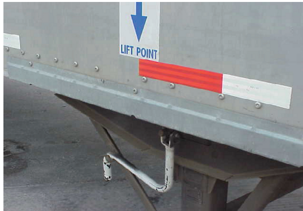
Fig. 4.6 Incorrect lift point
