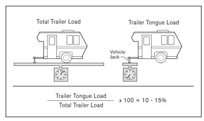
is placed directly under the trailer tongue coupler, and the tongue is set at the height/level of the tow vehicle hitch.
