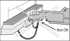
▲ WARNING- DO NOT use S-hooks for attaching the safety chains as they may become un-hooked while towing. If the S-hook unhooks, the emergency chains/cables will become detached, so if the tow hitch breaks or becomes disengaged, it will allow the trailer to completely break away causing property damage and possibly personal injury or death. The use of S-hooks is illegal in many states.
