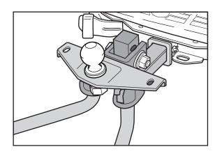
weight-distributing hitch ball mount (Class IV) is recommended if you plan to tow trailers with a maximum weight over 5,000 lbs. This ball mount includes a 2-5/16" hitch ball and is available through your NISSAN dealer.
