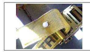
Re-install the ¼" nylon bolt and nut at end of the strap and hand tighten.
