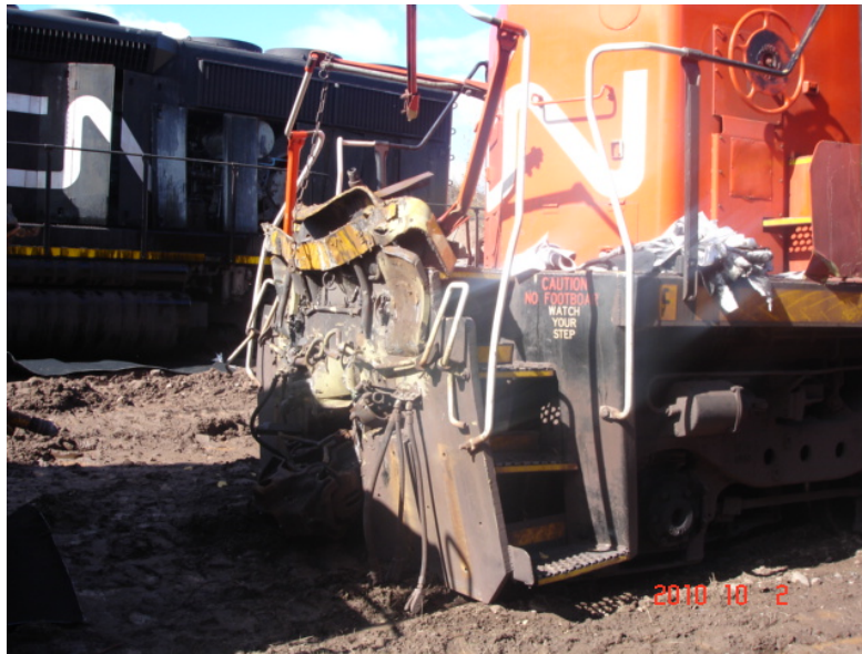
(a) Damage at the leading locomotive end.
