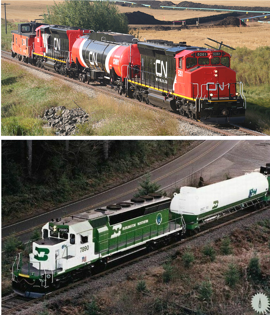
Figure 1. Photographs of the legacy LNG fuel tenders.
