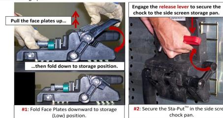
**#2**: Secure the Sta-Put<sup>™</sup> in the side screen chock pan.
