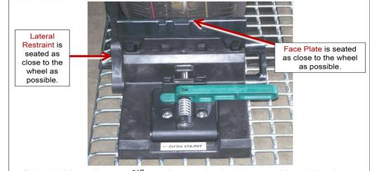
\* AAR Guidelines allow up to  $\frac{3}{4}$ " space between the chock device and the vehicle wheel.
