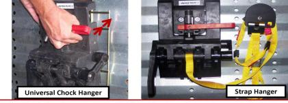
B) Secure the Strap: With J-Hook facing the side screen securely wind the strap onto the hanger, ensuring it does not lie on the railcar deck.
